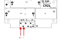
Connect the external power adapter (or any other regulated 12VDC power supply) to the power input of the connector:
